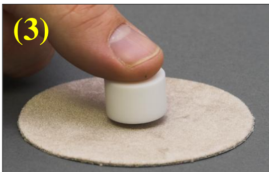
(3) Carefully push Teflon holder down until disk and holder surfaces are flush.
