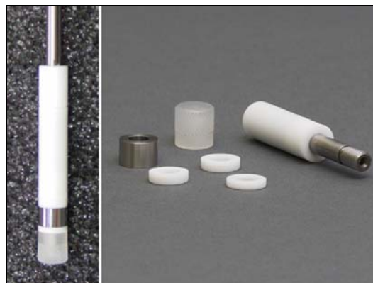
Figure 2: Rotating Cylinder Electrode Tip (easily taken apart to replace metal sample)
