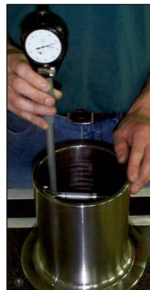
Figure IX: Use of Dial Bore Gauge to Probe SGC Mold Bore
