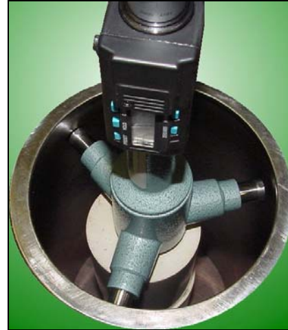
Figure VII: Use of a Three-Point Micrometer to Probe SGC Mold Bore (photographs courtesy of the Florida Department of Transportation)
