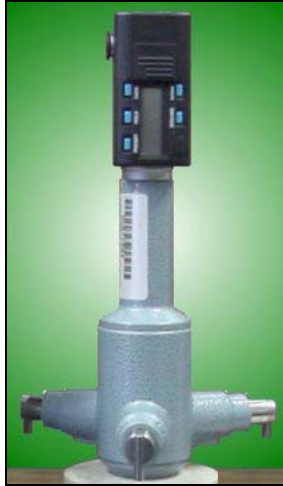
Figure VII: Use of a Three-Point Micrometer to Probe SGC Mold Bore (photographs courtesy of the Florida Department of Transportation)
