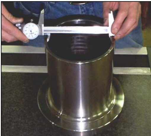
Figure VI: IMPROPER Mold Measurement Technique
